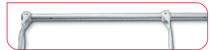
For use with infants and toddlers, the measuring rod has head and foot pieces that slide.
