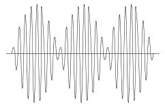
Figure 2—Premodulated Waveform
