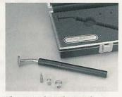
The optional Mettler Pencil Electrode has four interchangeable tips for maximum treatment versatility.
