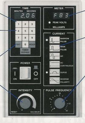
LED Displays indicate output intensity in peak volts or milliamps, and treatment time remaining.
