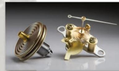
At the heart of every ADC aneroid is a movement assembled under optimum conditions to ensure it is free of the contamination found in lesser-built competitive instruments. The precision-crafted movement is heat treated and pre-aged to eliminate hysteresis, the stretching that often plagues cheaper products and knocks them out of calibration early in their life. The basic movement is optimized for each of the various models we produce.
