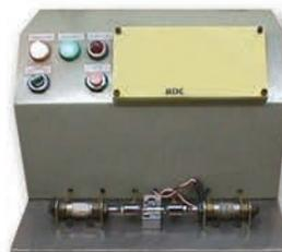
Valve-leak test machine
