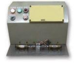
Valve-leak test machine
