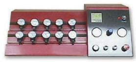
Gauge endurance test machine tests manometers to 30K cycles
